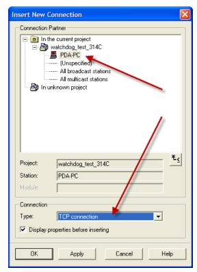
After the connection has been made, the properties of the created connection will pop-up. Here you can specify the port number and the name of this connection. In this example the port number 1501 is used. The block parameters you can see in this properties window are needed as input for the AG\_RECV in FC500. Check again if the ID and LADDR indicated here, match with the values used in the AGC\_RECV call in FC500.
