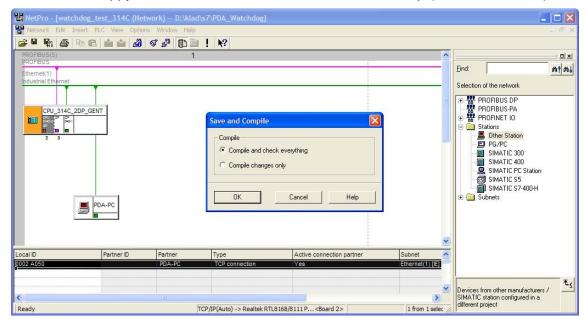
**8.** When the compilation finished without any errors, the configuration needs to be downloaded into the PLC. Click on the CPU of the PLC and afterwards click on the PLC icon where the arrow is pointing towards the PLC. Follow all the steps and reboot the PLC when asked for.
