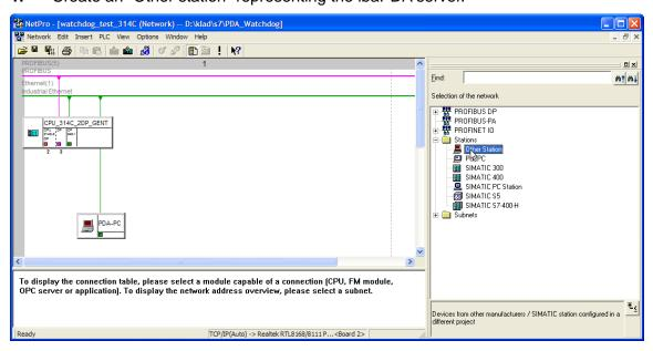
2. Rename the "Other station" to "PDA-PC" and assign it the existing S7 Ethernet connection.
