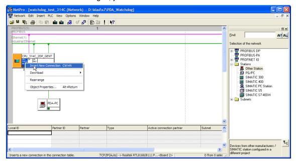
4. This new connection should be linked to the PDA-PC via Ethernet as configured in the screenshot below
